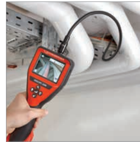
Inspection of hollow spaces
