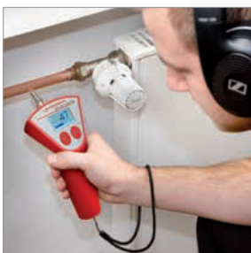
Acoustic Leak detection of heating installations
