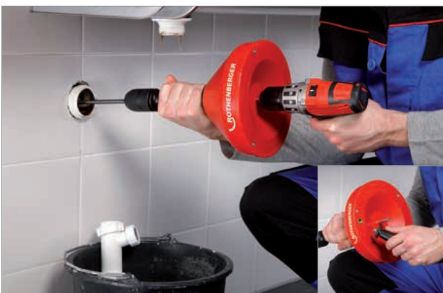
Electrical operation with cordless drill
