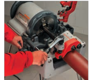
Cost-effective production of grooves
