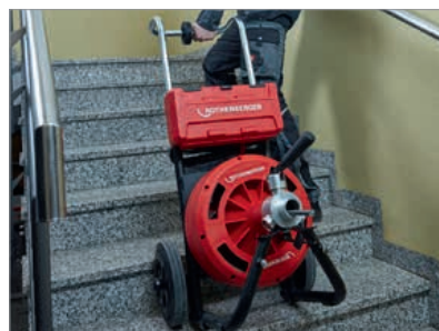
Easy transport due to stair capable chassis
