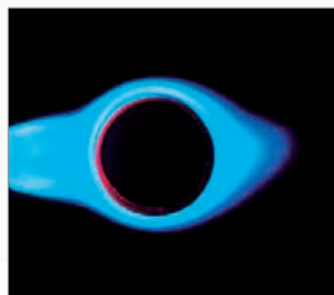
High flame temperature based on cyclone swirl
