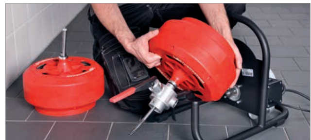
Interchangeable drum for different working ranges
